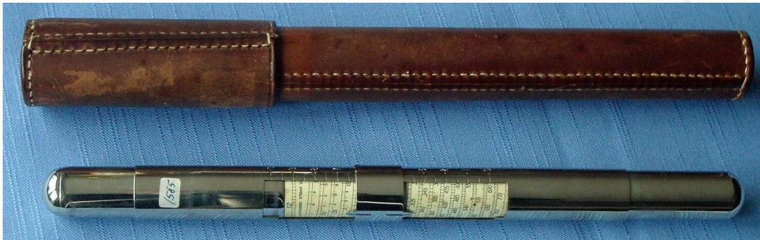
Fig. 15: Steward-made nickel-plated brass 9½ x Ø ¼ inch (50 inch helical scale) RHS Calculator
