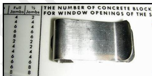
Fig. 3b: Concrete Calculator 's built-in metal “rule clip” (enlarged) fixed onto the back
