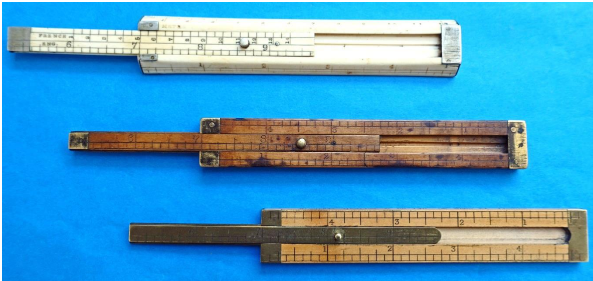
Three different Hat Rules or Gauges from my collection with their slides extended
