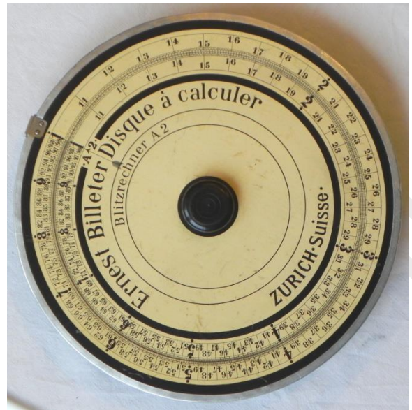
Figure 5: Billeter Ø 8 inch (21 cm) model A2 Blitzrechner with an effective scale length of 25.5 inches (65 cm)
