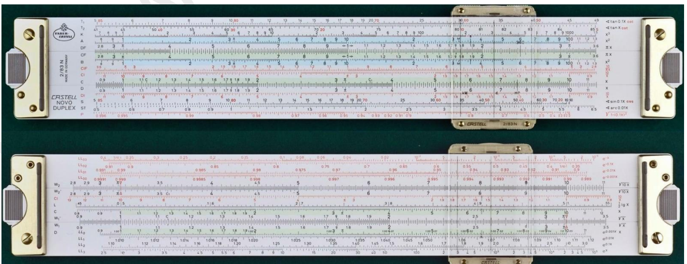
Figure 2: Faber-Castell 10-inch (25 cm) complex duplex model 2/83N with long scales on the back
