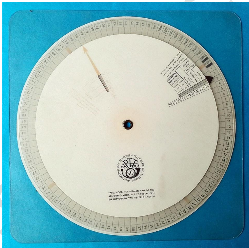
Fig. 2: ALRO plastic Ø 16.5 cm Time and Motion efficiency slide chart for the National Post Service in The Netherlands
