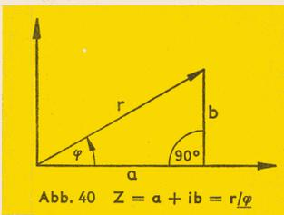
Abb. 40  $Z = a + ib = r/\varphi$
